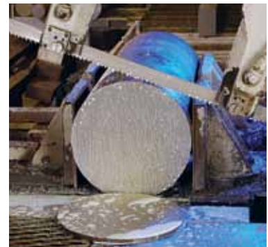
START TO CUT MATERIAL AT REDUCED CUTTING RATE
