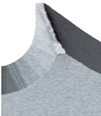
TOOTH INCORRECTLY BROKEN IN
