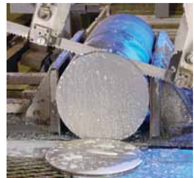
AFTER BREAK-IN WHEN THE BLADE HAS FULLY ENTERED THE WORKPIECE, INCREASE THE FEED RATE OVER A SERIES OF CUTS UNTIL THE RECOMMENDED CUTTING RATE IS ACHIEVED
