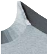
TOOTH INCORRECTLY BROKEN IN
