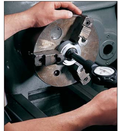
Above: Inspecting bore size with No. 84Z-111-4J.
