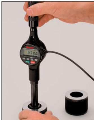
Using the No. 84Z-111-4J with No. F2710-1 Electronic Indicator to check hole size.
