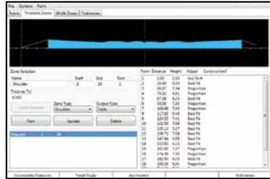
The design editor is tab driven, with tabs for Points, Thickness Zones, Width Zones, and Tolerances. Die break points are entered in the window shown at right, and can be imported as ASCII text characters. Note that all profile points must be entered first, and then the Zones are constructed from these points.
