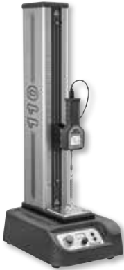
Shown: DFG mounted to FMM-110 digital test frame
