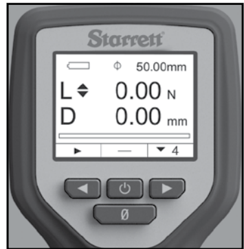
Shown: DFC displays both Load and Distance when connected to the FMM test frame.
