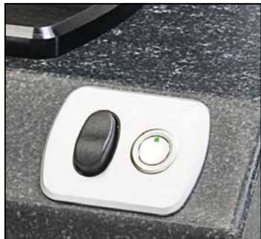
Jog Switch and Start/Stop Switch
