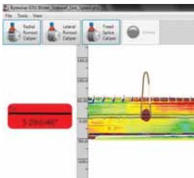
Figure 5 - Caliper Measurement Method
