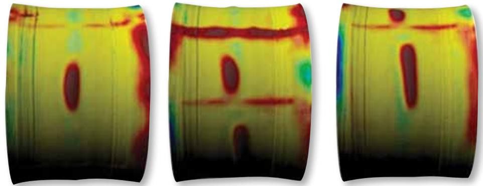
Figure 8- 3D Model Visualizations Showing Air Pockets between Inner Liner and Body Ply
