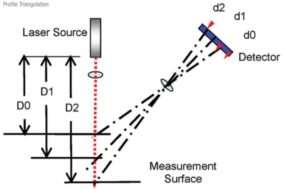
Figure 1 - Laser Triangulation Method
