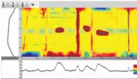
Figure 7- Entrapped Air Pockets between Inner Liner and Body Ply
