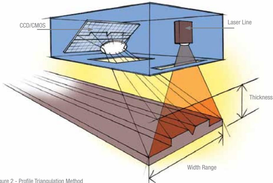
Figure 2 - Profile Triangulation Method
