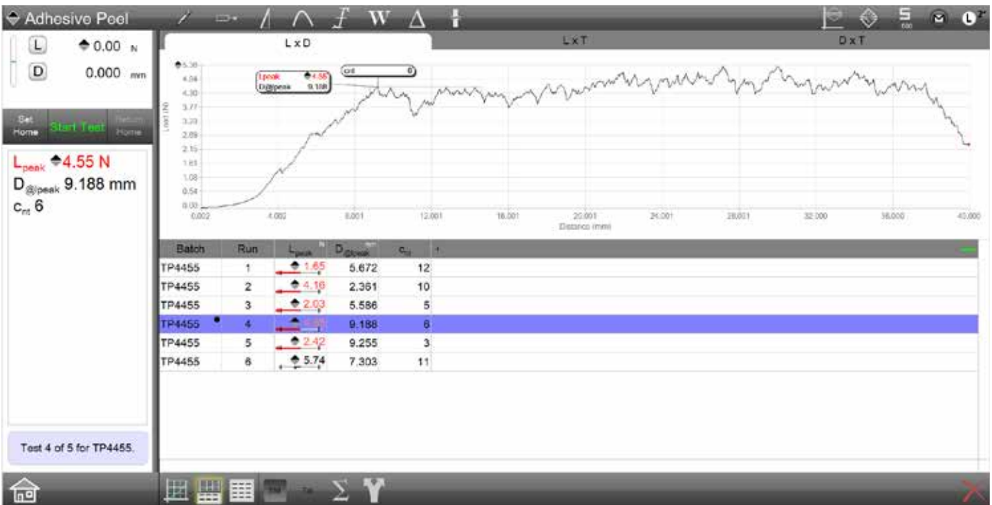
L2 Plus Full Graph view Adhesive test result showing graph trace and data view with tolerances
