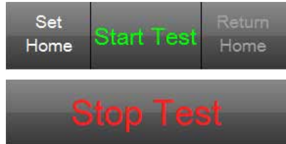
Start/Stop Test Soft Targets on Controller View
