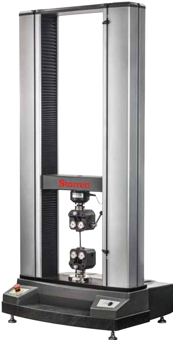
MMD-50K Series Testing Frame (50kN, 5000 Kgf, 11,250 lbf)
