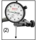
With the indicator attached, lock the pliers onto a stable structure.
