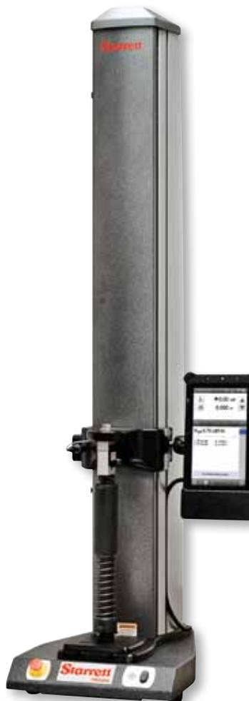
SMS Series spring testers come in four models based on their individual load capacities. They all use common software and load cell sensors. And with features such as a granite base, cast aluminum column and deflection compensation and linear error correction, they'll deliver reliable, repeatable load and length measurements.
