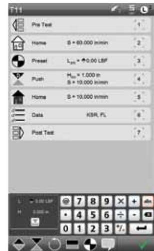
When the optional Test Builder software is installed, the user may convert a spring template and include more sophisticated test methods and advanced test results and reporting.
